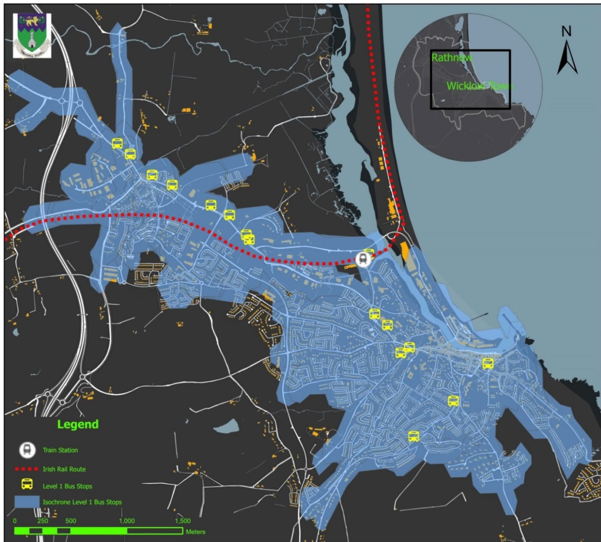
Map 15A: Level 1 Public Transport Stops (Train and Bus) 15 minute Isochrones Walking Time Map. A 'Level 1' Public Transport Stop is where there is more than 1 service route bus stop / train station operating at that stop.
